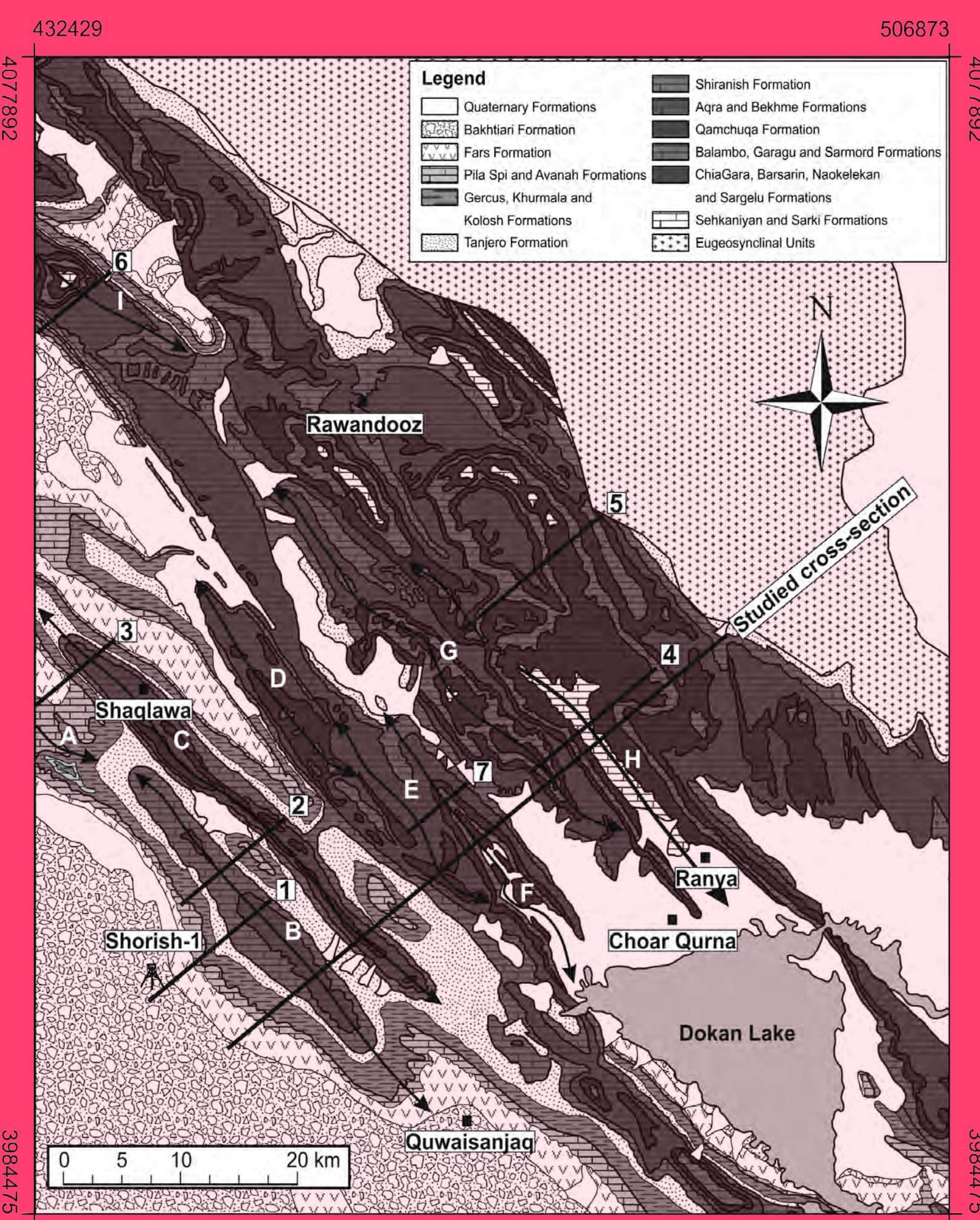
Geological map of the study area after Sissakian et al. (1997) with the positions of the 55.5 km long cross-sections. The shortening of several short balanced cross-sections is kinematically calculated as (1) 4.5%, (2) 14%, (3) 14%, (4) 15.3%, (5) 16.9%, (6) 14.6%, and (7) 13.5%, which shows an increasing deformation from SW to NE.
