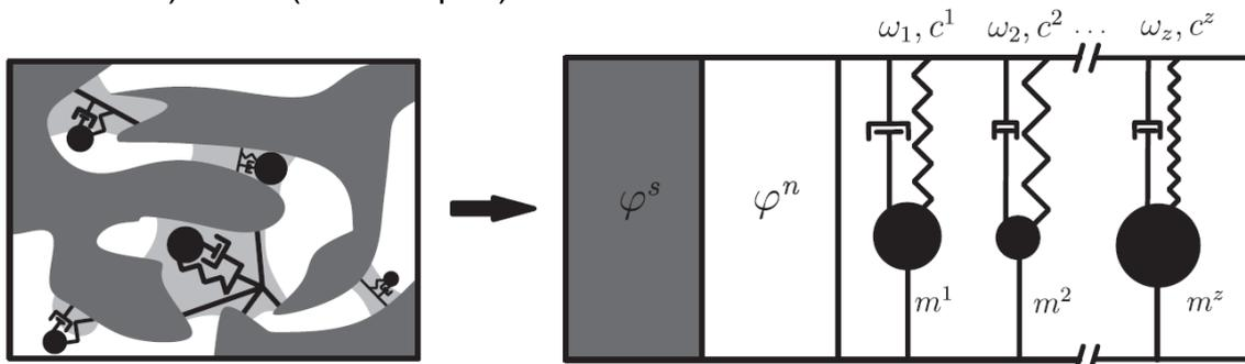
Figure 1. Upscaling from the heterogeneous pore-scale to an oscillatory behavior of the wetting blobs with different eigenfrequencies and damping mechanisms at the macroscale (REV). The extended poroelastic model with the continuous solid skeleton  $\varphi^s$ , the continuous non-wetting phase  $\varphi^n$  and the discontinuous oscillators representing the wetting phase  $\varphi^w$  is depicted.
